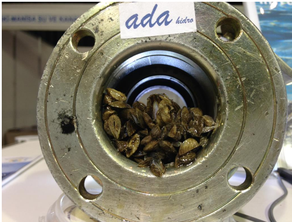
Figure 9. Zebra Mussel accumulation in a pipeline
