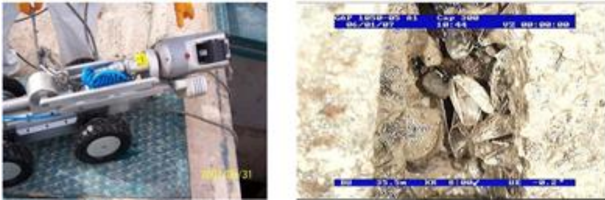
Figure 17. Robotic Camera and Zebra Mussels accumulation into the connection part of the pressured CTP type pipe (21).
